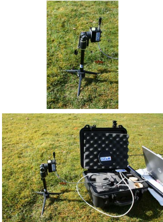
Figure 9: Pictures of the fibre and lens being set-up to take the 'Blue Sky' measurements.
