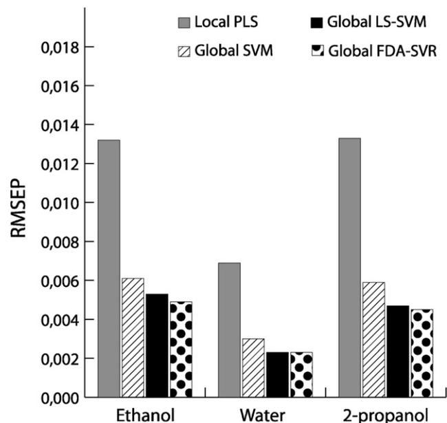
Fig. 3. Performance of different approaches together with the newly presented model based on FDA-SVR, for temperature influenced near-infrared dataset.
